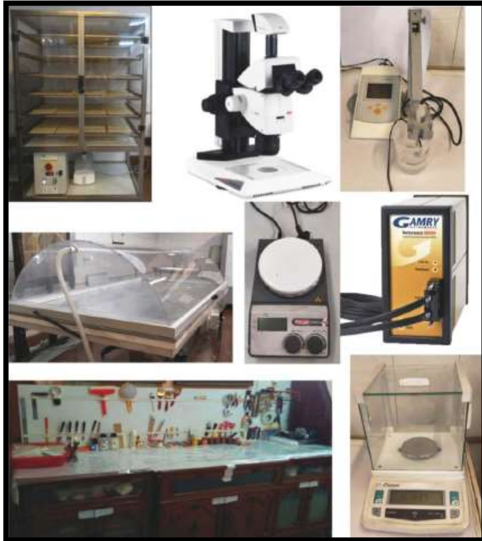
Fig.4: Photographs of some of the facilities of Conservation Division. First Row, L-R: Ultrasonic Humidifier, Stereomicroscope, pH meter. Second Row, L-R: Low Suction Table, Magnetic stirrer, Potentiostat. Third Row, L-R: Tool Table, Weighing Balance.
